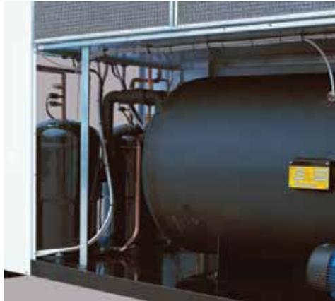
Unlike traditional chillers, Hyperchill places the evaporator stage within the tank, with the temperature control sensor positioned on the water outlet: this guarantees a very accurate water outlet temperature control. Water temperature stability is further improved thanks to the oversized water tank.
